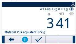
4 When the weight value is stable, press the checkmark to proceed with the next material of the formulation.
